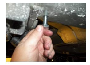
5. Raise hitch into position and insert (items 1 & 2) on driver's side, and (item 4 & 5) on passenger's side. Insert bolts through the bracket and frame as shown in Figure 1 for support. Note: The bumper locator pin may interfere with the hitch hardware. If necessary, use an angle grinder to trim the locator pin at the shoulder to allow proper hardware clearance.
