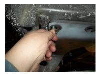
7. Install remaining conical washers and hex nut onto matching bolts.
