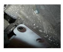
6. Insert M10 bolts (item 8 & 7) through bracket and into the frame as shown in Figure 1 (Hand tighten).
