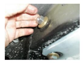
8. <u>Tighten M10 CL10.9 fasteners with torque wrench to 40 Lb.-Ft. (54 N\*M), both 1/2 GR5 fasteners with torque wrench to 75 Lb.-Ft. (102 N\*M) and M12 GR 8.8 fasteners with torque wrench to 68 Lb.-Ft. (92 N\*M).</u>
