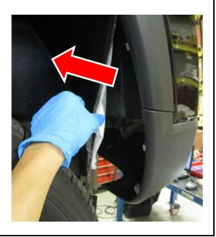
2. Enlarge access hole – peel off (3) plastic covers from holes on the frame rails each side, see <u>Figure 2</u>. Locate the rearmost hole and use die grinder to enlarge the hole size big enough to feed the bolt and spacer each side, see <u>Figure 2</u>. **NOTE:** for the models with factory tow hook, use 21 mm socket to remove M14 bolts in these locations and save them for reinstallation
