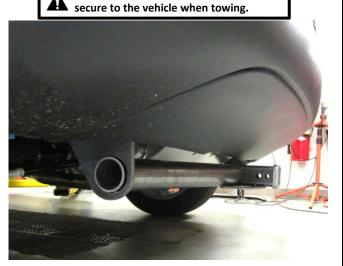
Proper torque is needed to keep the hitch
