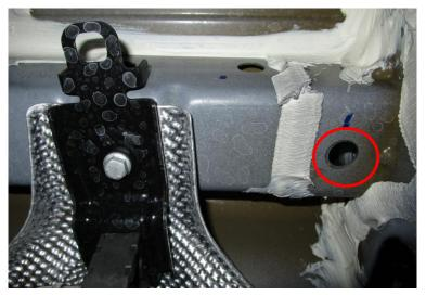
**3. Lower exhaust hanger and caulk removal** – use 13 mm socket to remove (1) bolt from exhaust hanger each side and lower the muffler temporarily, see <u>Figure 2</u>. Use a support or bungee cord to keep muffler from getting damaged. Use utility knife to remove caulk near rear mounting holes, see <u>Figure 3</u>. Bend down or cut off the legs of exhaust hanger bracket both sides for easier installation, see <u>Figure 3</u>.
