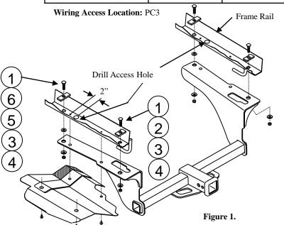
Equipment Required: Tin snips, Spray lubricant
